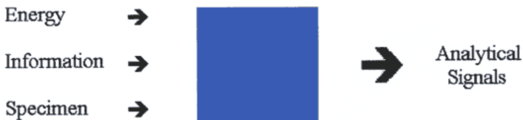
Figure 1. The functions of an analytical instrument.
